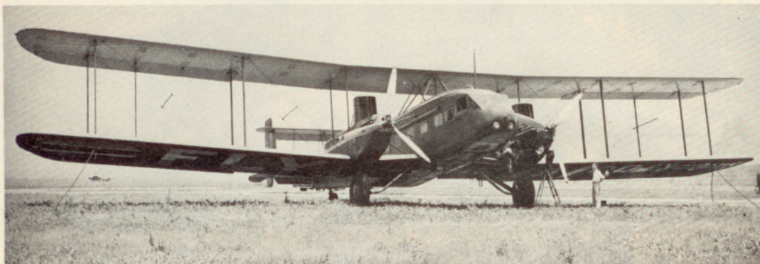
The first three Condor transports used the bomber wings, tail, and nacelles, but stretched the fuselage to accommodate a cabin for 18 passengers, two pilots, and a steward.
